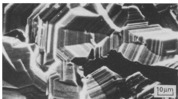
Fig. 2. Microphotograph of titanium crystal formed at melt/gas boundary in chloride-fluoride solvent mixtures.
